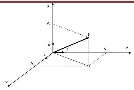
The modulus of the vector  $\vec{V}$  is :  $V = \sqrt{V_x^2 + V_y^2 + V_z^2}$
