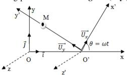
2- The relative acceleration  $\overrightarrow{a_r}$ , the entrainment acceleration  $\overrightarrow{a_e}$  and Coriolis acceleration  $\overrightarrow{a_c}$ , deduce the absolute acceleration  $\overrightarrow{a_a}$ .
