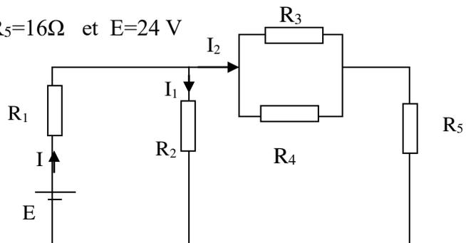
$$\frac{1}{R_{34}} = \frac{1}{R_3} + \frac{1}{R_4} = \frac{1}{6} + \frac{1}{12} = \frac{3}{12} \Rightarrow R_{34} = 4\Omega \text{ (0.25pts)}$$
