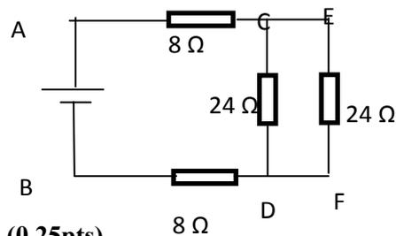
$$\frac{1}{R_{eq4}} = \frac{1}{24} + \frac{1}{24} = \frac{2}{24} = \frac{1}{12} \text{ donc } R_{eq4} = 12 \Omega \text{ (0.25pts)}$$
